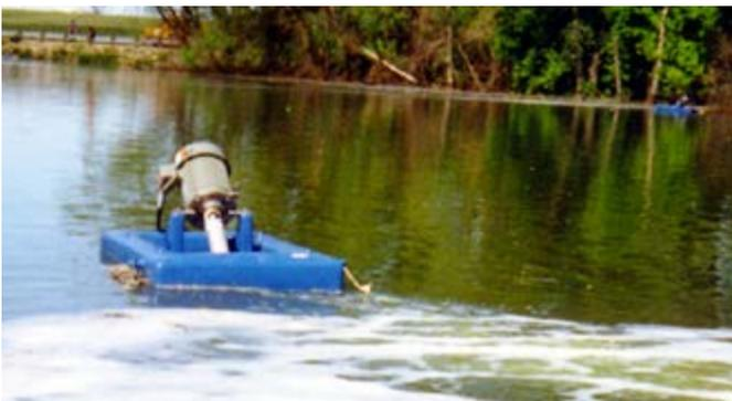
The Aqua Tornado injects air into the water at a high velocity at the open propeller hub. The turbulence and flow created by the propeller breaks-up the air bubbles, mixes, and disperses oxygen over a wide area. The horizontal water movement greatly limits algae growth, while stimulating decomposition of organic wastes and runoff nutrients from surrounding green areas. Aeration quietly occurs just below the surface with no spraying or splashing, reducing odors.
